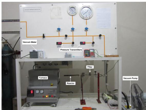
**Figure 1.** A schematic of the homemade Sievert's type apparatus which is used in our studies.
