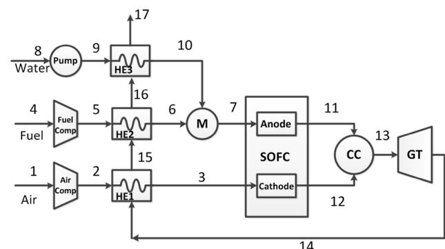
Fig. 1. Schematic of standard SOFC-GT hybrid system
