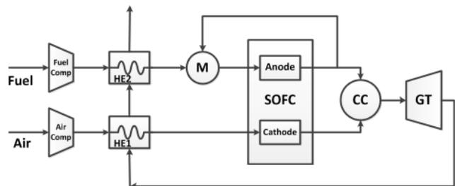
Fig. 9. Schematic of hybrid system with the anode products recycling.
