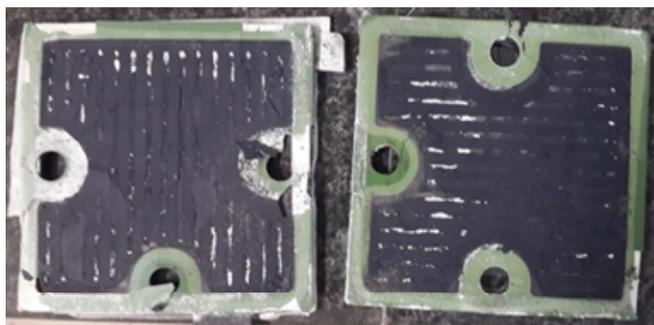
Fig.6. Image showing the two cells used in the stack after operation.
