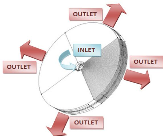
Fig. 2. Schematic of the radial fuel cell
