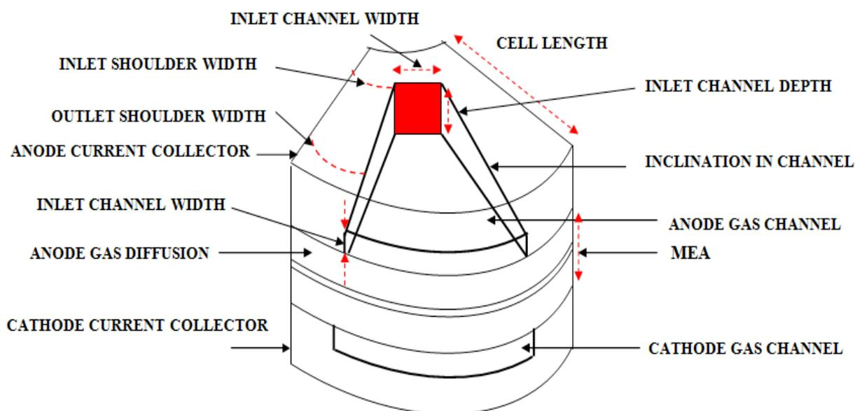
Fig. 3. Simplified model of the radial fuel cell
