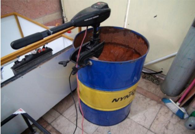
Fig. 10. The boat motor as the system load.
