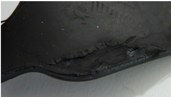
Fig.13. Changes in the appearance of the silicone sealant.
