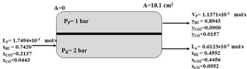
Fig. 3. Modeling results of a single stage of silica membrane for hydrogen separation
