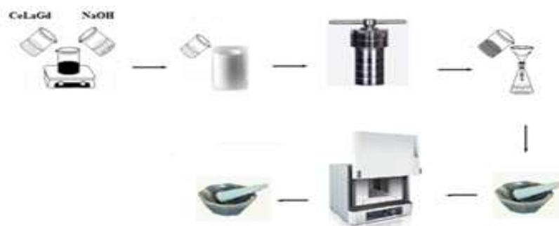
Fig. 1. Flow chart of hydrothermal method
