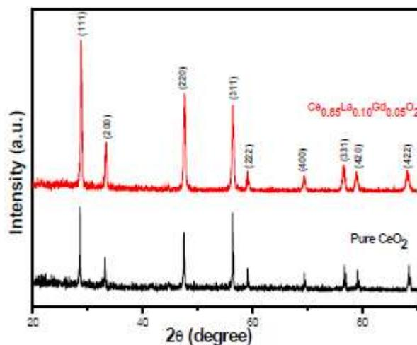
Fig.2 XRD of pure  $\text{CeO}_2$  and  $\text{Ce}_{0.85}\text{La}_{0.1}\text{Gd}_{0.05}\text{O}_2$  powder
