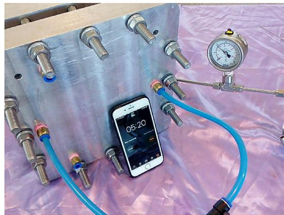
Fig. 2. Leakage test at pressure of 3 barg.
